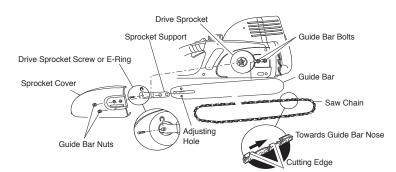
Figure 4 - Assembling Guide Bar and Chain
